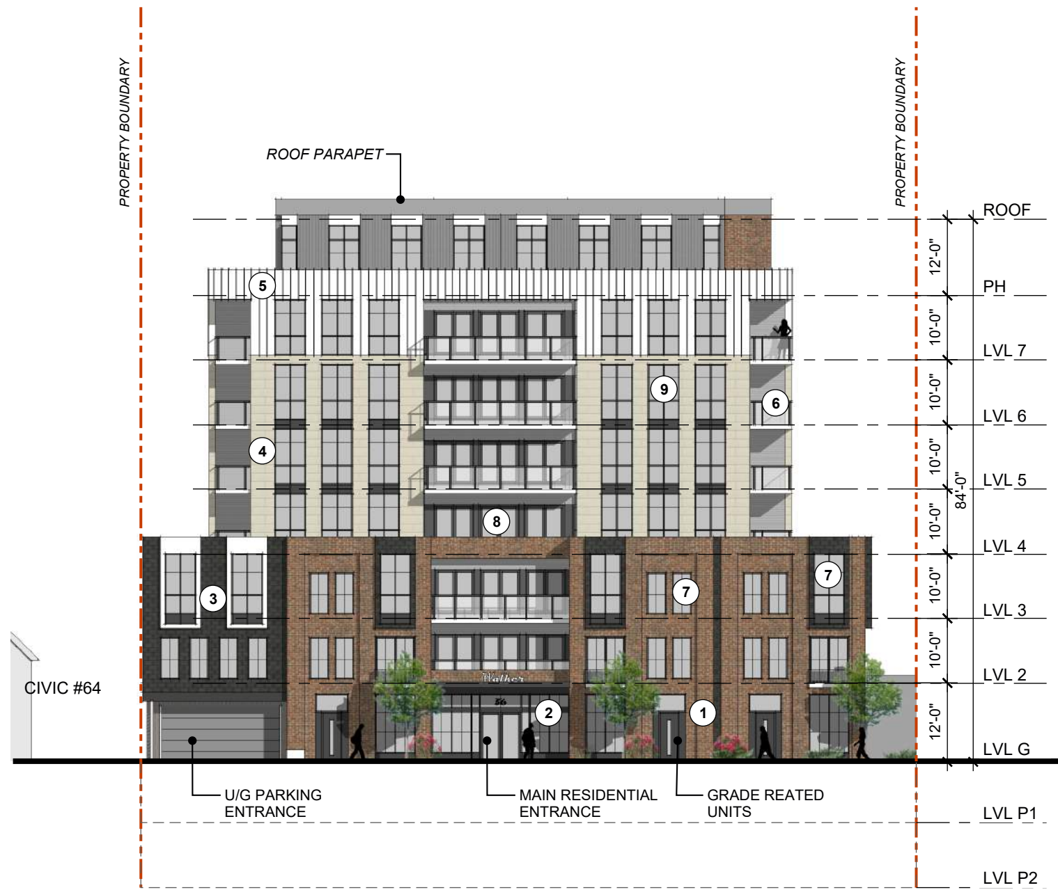
WEST ELEVATION (FRONT)
